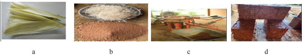
Fig. 2. Materials used for the experimentation: a) corn husk waste, b) soil and corn husk fibers, c) compression moulding machine, d) block obtain after moulding for drying
